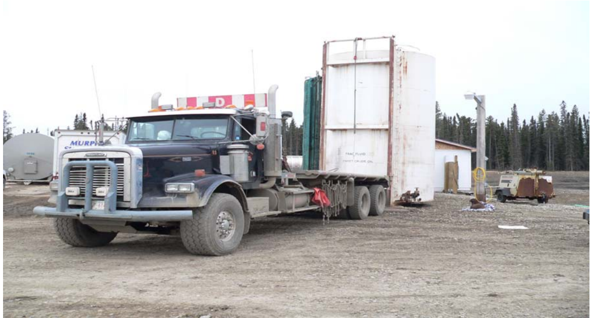
Photograph #1 Shows the truck involved in the incident. The operator was backing up to the tank. The tank was to be loaded on to the bed truck and moved to another location in the yard.
