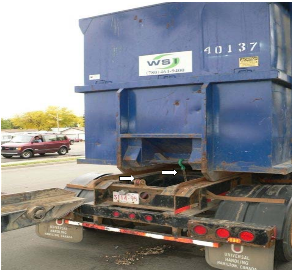
Photograph #5 Shows the rear of the trailer that the Senior Worker was pinned against. The arrows identify a portion of the hold down mechanism that he was unsecuring at the time of the incident.
