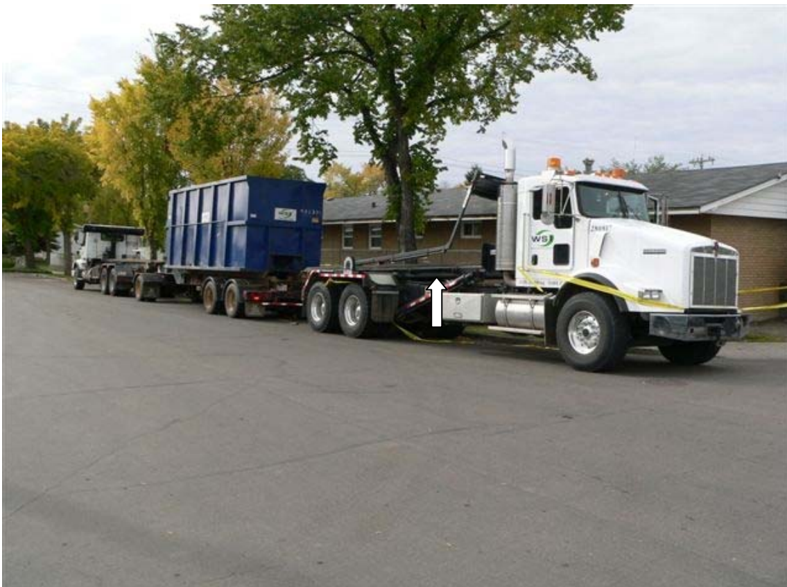
Photograph #1 Shows the scene with the Kenworth truck on the right of the photograph and the truck/trailer unit with the blue garbage bin on top of the trailer behind the Kenworth truck. The arrow identifies one of the slightly elevated rails; its hydraulic lifting ram is identified by red and white reflective tape just behind the arrow.
