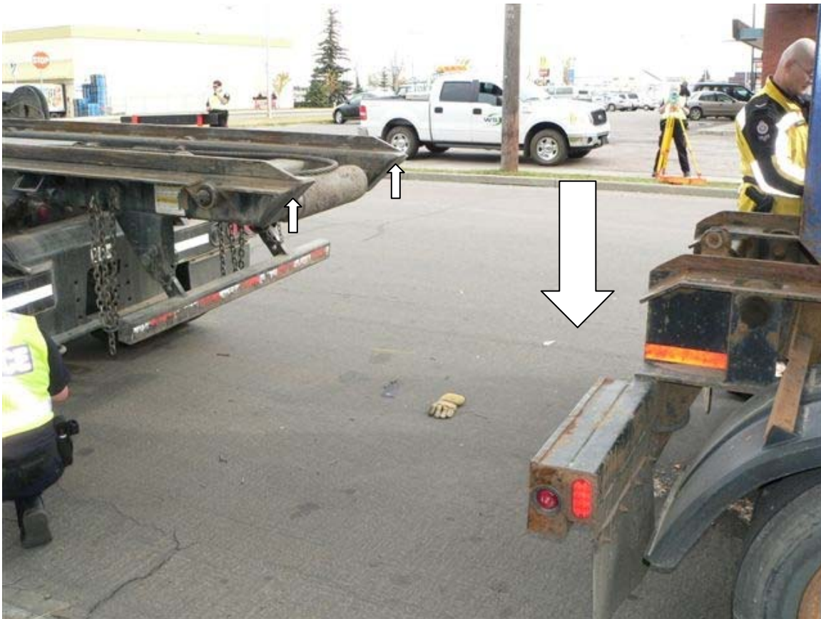
Photograph #4 Identifies the rear of the Kenworth truck on the left of the photograph with the rear of the trailer secured to the truck the Senior Worker was operating visible on the right of the photograph. The large arrow identifies the location where the Senior Worker was standing when he was contacted and pinned by the Kenworth truck. The small arrows identify the ends of the rails that are placed under the garbage bin to facilitate the transfer when the rail mechanism is tilted.
